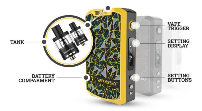
A mod is the term by which a vaper describes the vaping "device" as a whole but, more specifically, its electronic / battery component.
