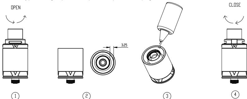
5. **Changing Atomizer:** Unscrew the base to simply remove and insert a new atomizer whenever needed. Pull the EUC out from the base and insert a new one. Screw the Base on. Wait after replacing to make sure the coil is well primed.
